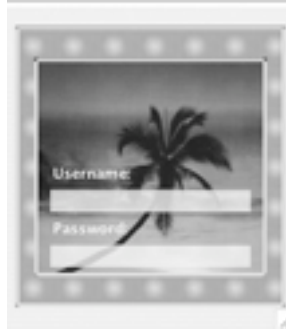
Fig. 2. The trusted password window displays a visual hash that should match the website image
